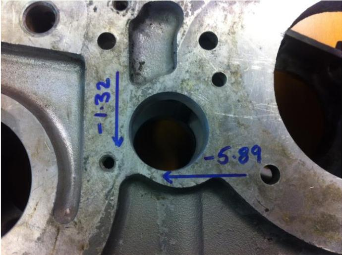
Clean the inner face again using the custom tool until flush with the prior machined face.
