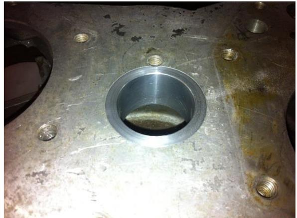
Apply a small amount of locktite to the rear of the tabbed thrust washer and lay the washer on the newly machined inner face of the small pin bush (the locktite is used for ease of assembly when installing the internals)
