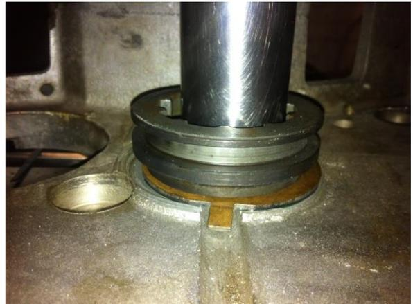
Once the locktite has set remove the pin and weight, there is a threaded hole that get broken into when boring the large pin hole. Run a tap through this hole to restore it back to normal. The thread is 3/8 UNC x16.
