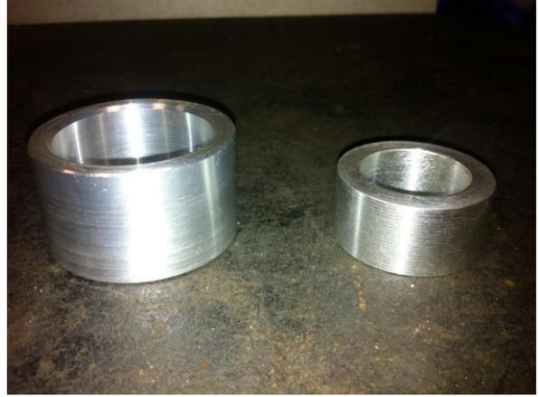
The pin bushes should both be a transition fit (sliding fit) on the centre pin and into the newly machined casing, apply a generous amount of bearing locktite onto the outer of the pin bushes and insert them into the corresponding holes in the machined casing ensuring they sit flush with the casing outer.
