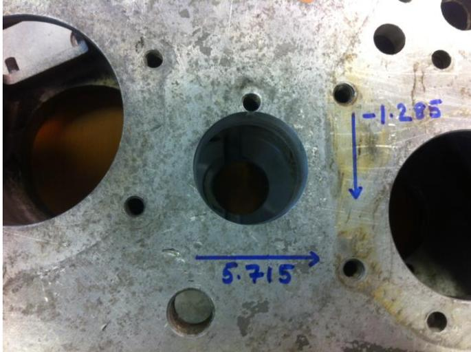
We need to now clean up the inner face of the bore whilst the machine is centered to accept the supplied tabbed thrust washer, for this procedure we use a custom back cutting tool and skim the inner face flush to the prior machined face as shown below.
