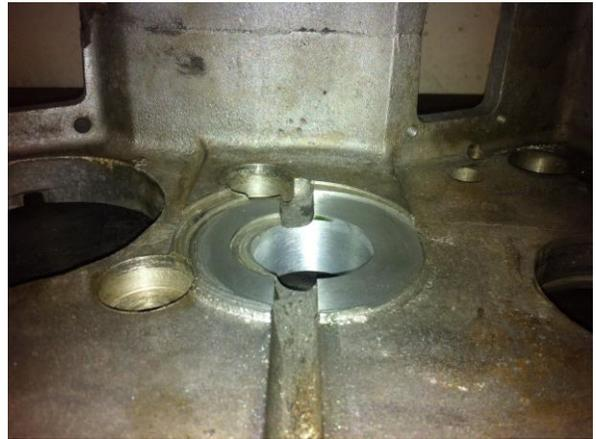
Turn the casing over so the small pin hole is now facing upwards, square the flat of the casing with the bed of the milling machine and centre the small pin hole as described before.
